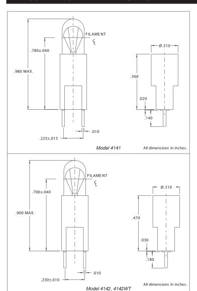
Mounting: Printed circuit Board
