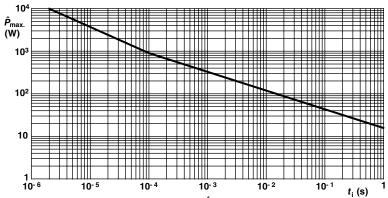
Pulse on a regular basis; maximum permissible peak pulse power  $\hat{P}_{max}$  as a function of pulse duration (t) for single pulse condition
