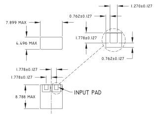
NOTE: RESONATOR HOLES NOT SHOWN. ALL DIMENSIONS IN MM.
