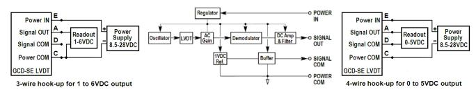
A through E: Connector pin assignments
