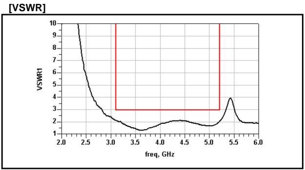
Note: Tested antenna has been soldered on 24X43mm<sup>2</sup> PCB.
