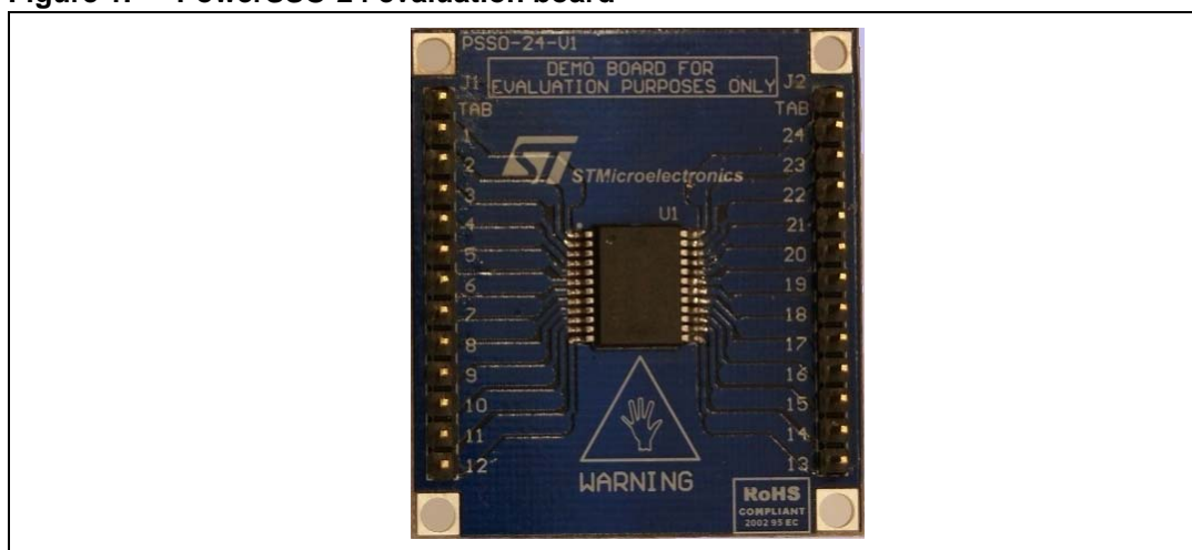
Figure 1. PowerSSO-24 evaluation board
