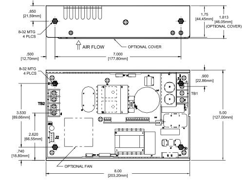
A. Units should be allowed to warm up/operate under non-condensing conditions before application of power. Derate output current and total output power by 2.5% per °C above  $50^{\circ}$ C.
