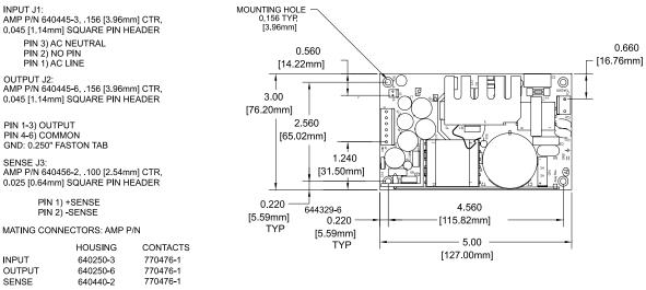
MAX. COMPONENT HEIGHT1.20" [30.28 mm] MAX. LEAD PROTRUSION 0.10" [2.54mm]
