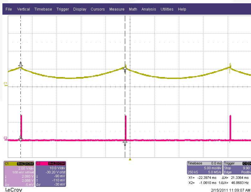
Figure 1. 264V / 60Hz at No Load
