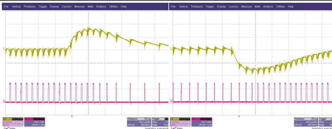
Figure 14. FAN6754AMR 230V / 50Hz, Overshoot (Ch1: V OUT , Ch2: Gate)
