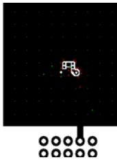
c. 110 °C/W when mounted on a 1 in 2 pad of 2 oz copper.
