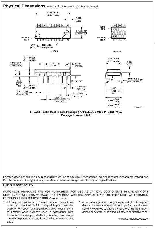
DM74S140 Dual 4-Input NAND 50<sup>Ω</sup> Line Drive
