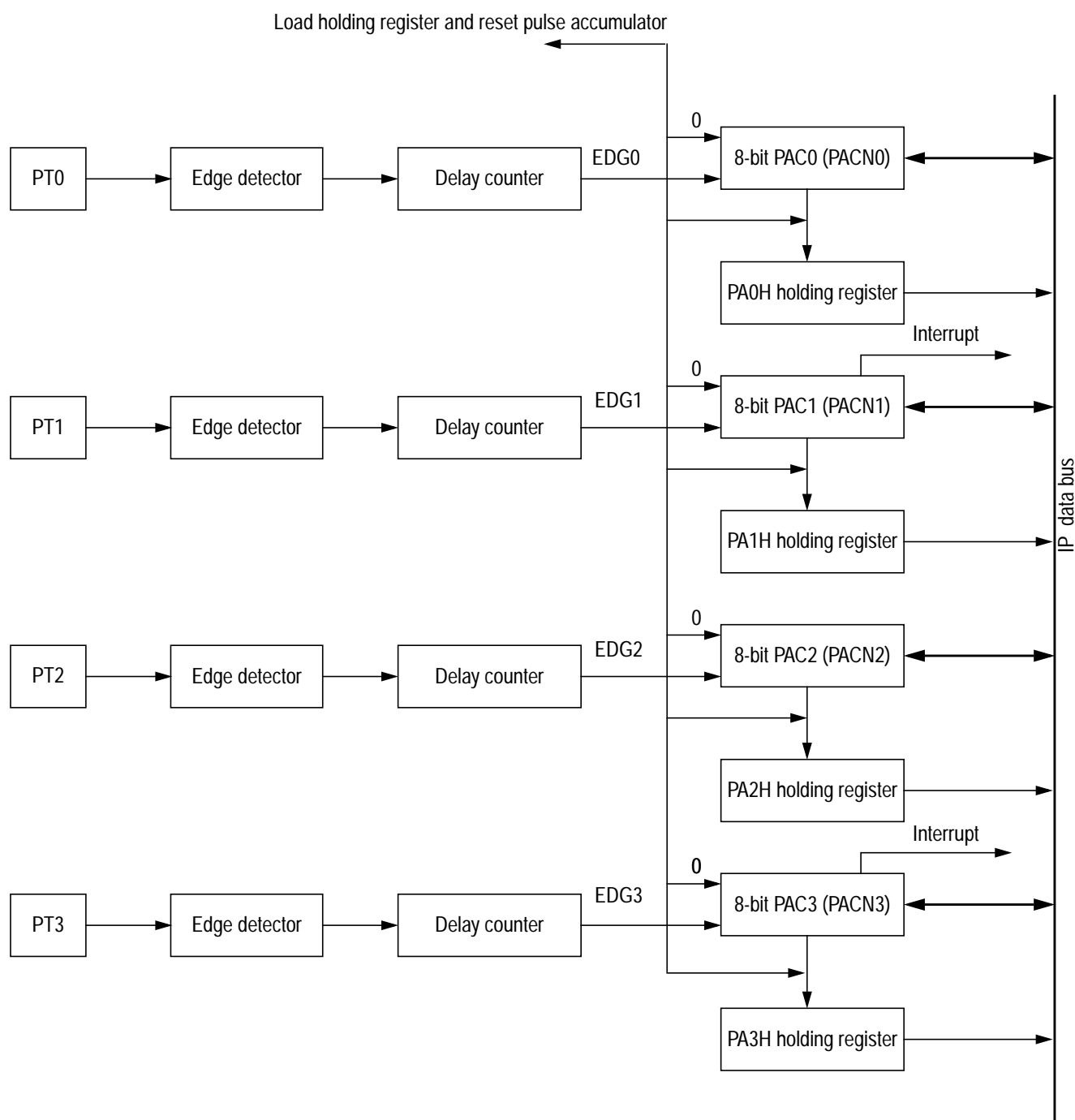
Figure 71 8-Bit Pulse Accumulators Block Diagram
