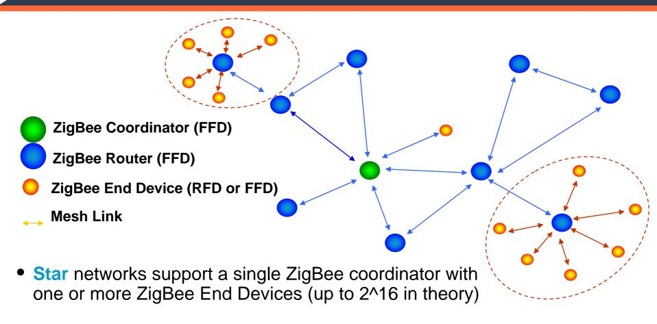
Mesh network routing permits path formation from any source device to any destination device
