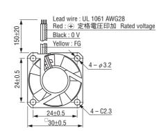
取付穴参考寸法 Dimension of mounting hole for recommendation
