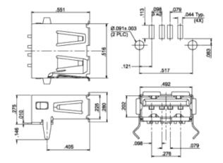
Description: USB Socket Type A Single Row Surface Mount Plating Code: 30 Shell Plating: N/A
