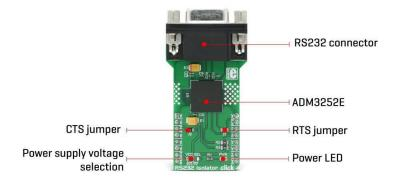
Besides the UART RX and TX lines, the click also supports the hardware flow control via the CTS and RTS lines. One of the two existing channels is used for the UART data communication itself, while the other channel is used for the hardware flow control lines. The usage of the control lines is not always mandatory, so the lines can be disconnected from the mikroBUS if needed, by unsoldering the SMD jumpers labeled as J1 and J2.
