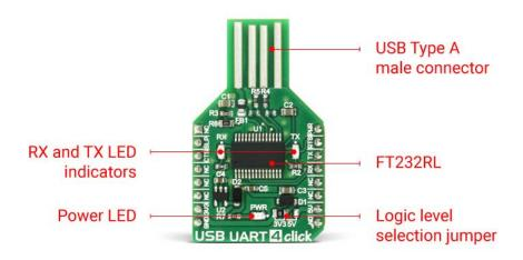
This device also features the configurable CBUS pins, which can be used for several different useful functions, as for example - configurable clock out for driving the microcontroller, data LED drive, USB Sleep, PWR status and so on. By default, CBUS3 and CBUS4 pins are configured as Power Enable and Sleep options and are routed to the PWR and SLP pins of the mikroBUS<sup>TM</sup>. More information about configuring the CBUS pins can be found in the FT232RL datasheet.
