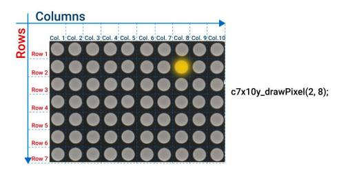
• void c7x10y\_drawText( char \*text )- Writes the text; The first character is placed on the first LED matrix, and the second one is placed on the second LED matrix (if a there is more than one character).
