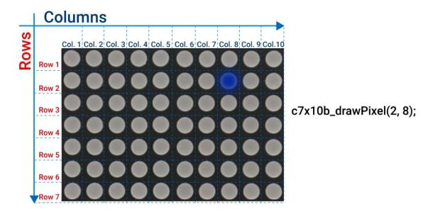
• void c7x10b\_drawText( char \*text )- Writes the text; The first character is placed on the first LED matrix, and the second one is placed on the second LED matrix (if there is more than one character).
