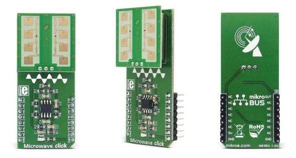
**Microwave click** detects movement, thanks to the PD-V11 a 24GHz microwave motion sensor. The typical use for Microwave click is a proximity or motion detector in various applications and devices.
