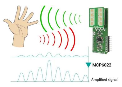
The PD-V11 microwave motion sensor low power consumption, low noise, and a low wireless power output. See the datasheet to learn more. https://download.mikroe.com/documents/datasheets/PD-V11.pdf
