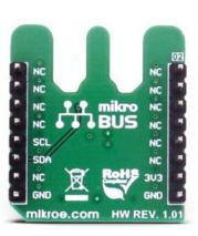
**Thermo 6 click** is a precise and versatile ambient temperature measurement click board<sup>TM</sup>, based on the Maxim Integrated MAX31875 temperature sensor. This sensor has a great combination of features, such as wide range of temperature measurement, excellent measuring accuracy, and small die size, coupled with the very low power consumption - attributes that make this sensor a great choice for many different applications.
