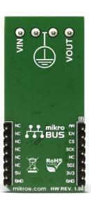
MCP16331 click functions as a non-inverting buck-boost voltage regulator, a type of switching mode power supply topology that combines the principles of the Buck converter (step-down) and the Boost converter (step-up) in a single circuit.
