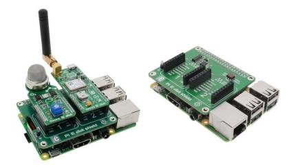
Picture on the right shows Pi 3 click shield connected to the Raspberry Pi® 3 model B, picture on the left shows the connected shield along with two click boards<sup>TM</sup>: Ozone 2 and GNSS 5 click.
