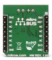
**1-Wire I2C click** carries DS28E17 1-Wire-to-I2C master bridge from Maxim Integrated. The click runs on a 3.3V power supply.
