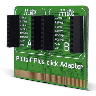
**PICtail™ Plus click Adapter** allows you to add click boards™ on the Explorer 16 Development Board from Microchip. It's an adapter with two mikroBUS™ sockets for click board connectivity.
