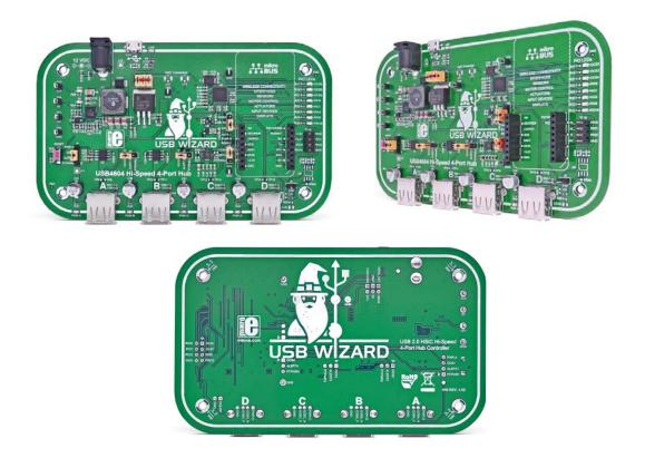
**USB Wizard** is an evaluation and demonstration platform featuring the USB4604 USB 2.0 4-Port hub controller. The board has four USB 2.0 downstream ports with individual port power control and overcurrent sense (OCS).
