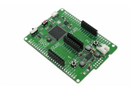
**Clicker 2 for MSP432** is a compact development board with two mikroBUS<sup>TM</sup> sockets for click board connectivity. It carries the SimpleLink<sup>TM</sup> MSP432<sup>TM</sup> - ARM® 32-Bit Cortex®-M4F CPU with integrated 1Msps 14-bit SAR-based ADC from **Texas Instruments**.
