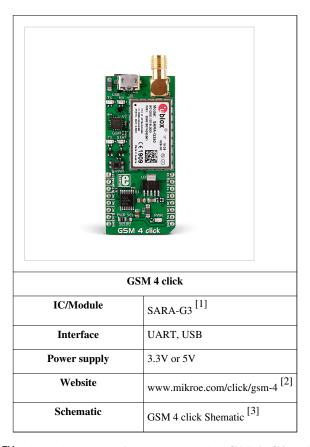
**GSM 4 click** is a mikroBUS<sup>™</sup> add-on board that features the u-blox **SARA-G3** series 2.5G GSM/GPRS cellular module. The SARA-G3 module has a miniature LGA (Land Grid Array) form factor as well as a RF transceiver and a power amplifier. The click can respond and react to phone calls or messages and send and receive data.
