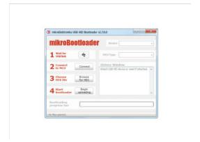
To start, connect the USB cable, or if already connected press the Reset button on your mikromedia plus for FT90x. Click the Connect button within 5s to enter the bootloader mode, otherwise existing microcontroller program will execute.
