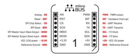
mikroBUS<sup>TM</sup> host connector consists of two 1x8 female headers containing pins to be most likely used in the target add-on board. There are three groups of communication pins: SPI, UART and I2C. There are also single pins for PWM, Interrupt, Analog input, Reset and Chip Select. Pinout contains two power groups: +5V and GND on one header and +3.3V and GND on the other 1x8 header. mikroBUS<sup>TM</sup> host connector perfectly fits into standard breadboards.
