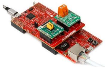
Click BoosterPack 2 is an extension for Texas Instruments LaunchPads<sup>TM</sup> with the current BoosterPack Pinout Standard. It has two mikroBUS<sup>TM</sup> sockets onboard, for simple and easy integration of **MikroElektronika click boards** with a LaunchPad<sup>TM</sup>.
