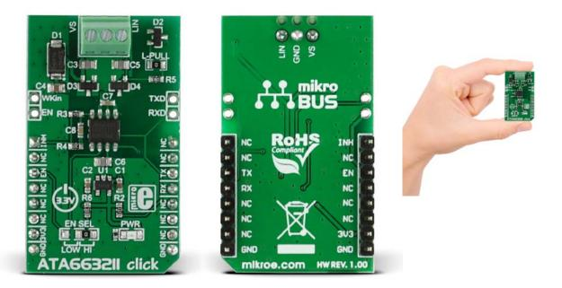
**ATA663211 click** carries an Atmel LIN transceiver IC designed to handle low-speed data communication in vehicles and in industrial applications with electrically harsh environments. The LIN connection is established by attaching wires to the onboard screw terminals.
