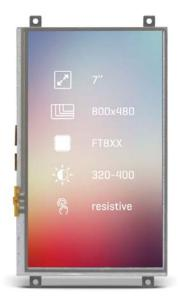
The **800x480px** screen is driven by an **FT812** graphic controller which is supported in Visual TFT, the GUI design tool for rapid development of user interfaces.
