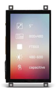
The **800x480px** screen is driven by an **FT813** graphic controller which is supported in Visual TFT, the GUI design tool for rapid development of user interfaces.
