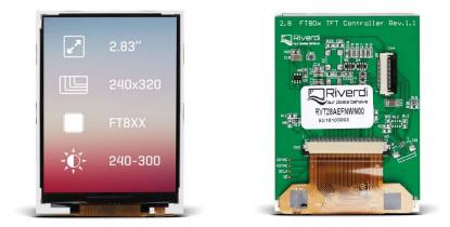
The **240x320px** screen is driven by an **FT800** graphic controller which is supported in Visual TFT, the GUI design tool for rapid development of user interfaces.
