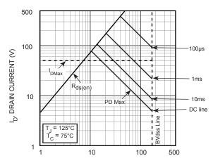
$V_{DS}$ , DRAIN-TO-SOURCE VOLTAGE (V) FIGURE 4, Forward Safe Operating Area
