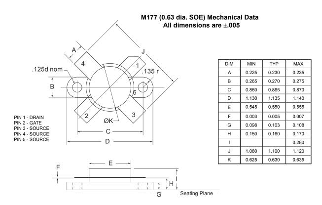
**HAZARDOUS MATERIAL WARNING:** The ceramic portion of the device below the lead plane is beryllium oxide. Beryllium oxide dust is highly toxic when inhaled. Care must be taken during handling and mounting to avoid damage to this area. These devices must never be thrown away with general industrial or domestic waste. BeO substrate weight: 0.703g. Percentage of total module weight which is BeO: 9%.
