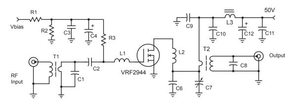
C1 1200pF ATC100B ceramic C2, C3 0.1uF 100V 1206 SMT C9-C11 .047uF NPO 100V 1218 SMT C6 180 pF metal clad mica C7 ARCO 465 mica trimmer C8 100 pF ATC 100E ceramic C4, C12 10uF 100V Electrolytic L1 25 nH - 2t #18 0.2"d .2"l L2 26 nH - 1.5t #12 0.31"d2 L3 2t #16 on 2x 267300081 .5" bead R1-R2 1k  $\Omega$  1/4W R3 100  $\Omega$  1W T1 16:1 transforner 4t #24 teflon on RF Parts Co. T1/2 transformer core T2 9:1 transformer 3t 2-ply #16 teflon on RF Parts Co. T1 transformer core
