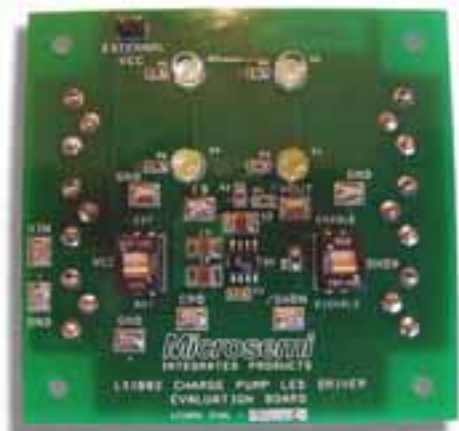
Figure 4. LX1882 LED Driver Evaluation Board (Top View)
