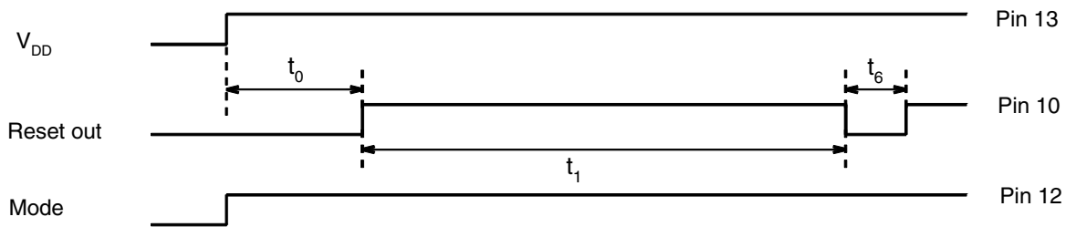
Figure 4-2. Power-up Reset and Mode Switchover
