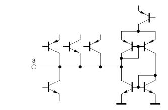
Figure 7-3. Internal Reference Voltage (Pin 4)
