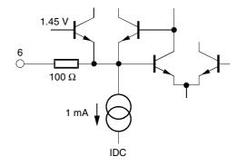
Figure 7-6. AGC Switch (Pin 7)
