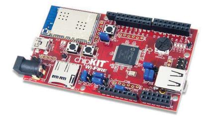
Building on the previous successes with the chipKIT WF32, the Wi-FIRE uses the same 43 available I/O pins, 12 analog inputs, 3.3 operating voltage, 4 user LEDs, potentiometer, buttons, uses MRF24 on-board wireless module, microSD Card, dedicated SPI Signals and high efficiency switching 3.3V switching power supply for low-power operation. Where the boards differ is in what the PIC32MZ processor can deliver.
