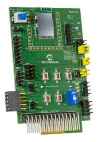
The RN-4870-SNSR is a development board based on the ultra-compact Bluetooth 4.2 Low Energy RN4870 module. The RN4870 uses a simple ASCII command interface over the UART. The board enables evaluation of the RN4870 and development of Bluetooth low Energy applications in two different ways:
