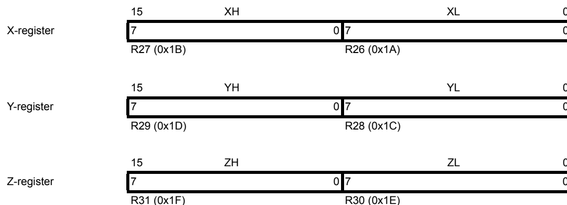
Figure 13-3. The X-, Y-, and Z-registers
