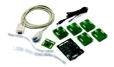
The ICE 200 is controlled by AVR Studio, the Integrated Development Environment (IDE), for developing and debugging AVR applications in a Windows® 95/98 or Windows NT® environment. The ICE 200 gives the user full run time control, unlimited number of breakpoints, symbolic debugging and full memory and register visibility.
