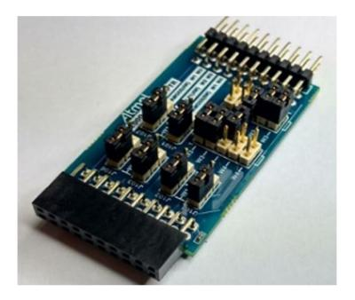
The Atmel® ATBTLC1000-XPRO-ADPT is an adapter board for the ATBTLC1000-XPRO expansion board. It is required for the UART hardware flow control functionality to operate correctly when the ATBTLC1000-XPRO expansion board is connected to certain Atmel Xplained MCU base boards.
