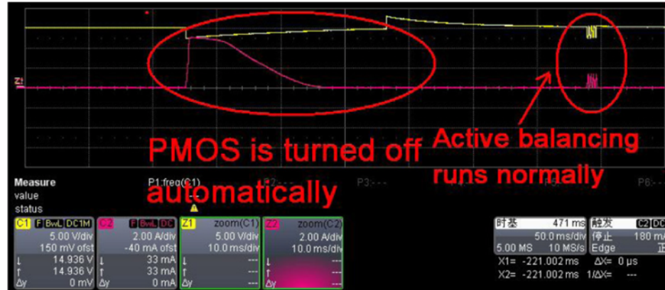
Figure 4-3. PMOS is Switched Off Automatically
