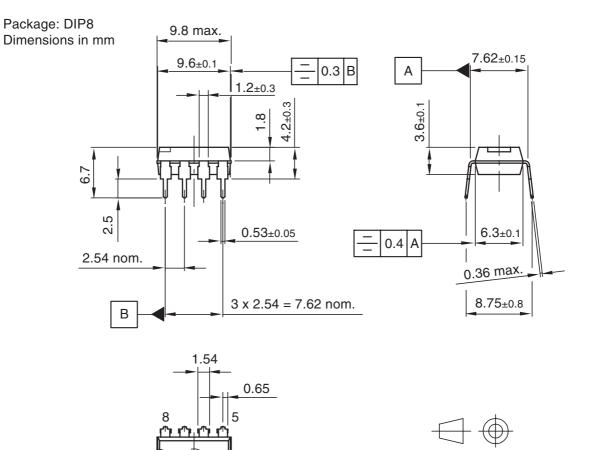
technical drawings according to DIN specifications
