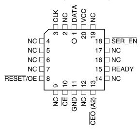
Notes: 1. 20-lead PLCC (Virtex® pinout) is only available in the AT17F040.
