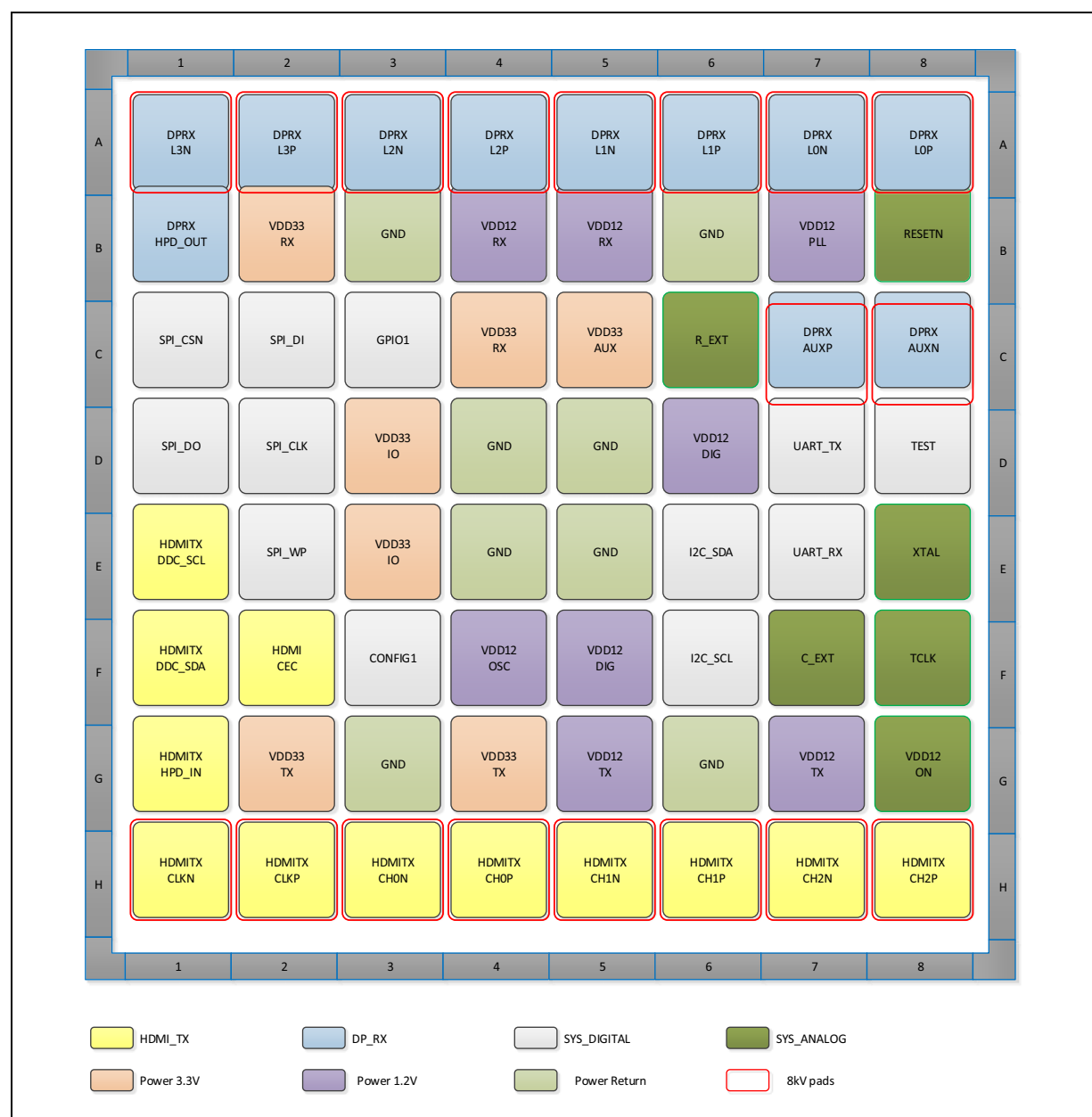
Figure 4. MCDP28x0 BGA diagram
