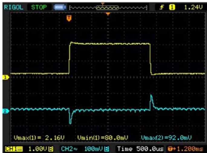
Figure 6. Transient response when load steps from 200mA to 2A in PWM MODE.
