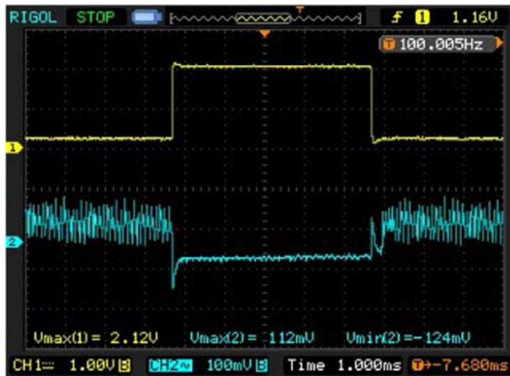
Figure 8. Transient response when load steps from 200mA to 2A in PFM MODE.
