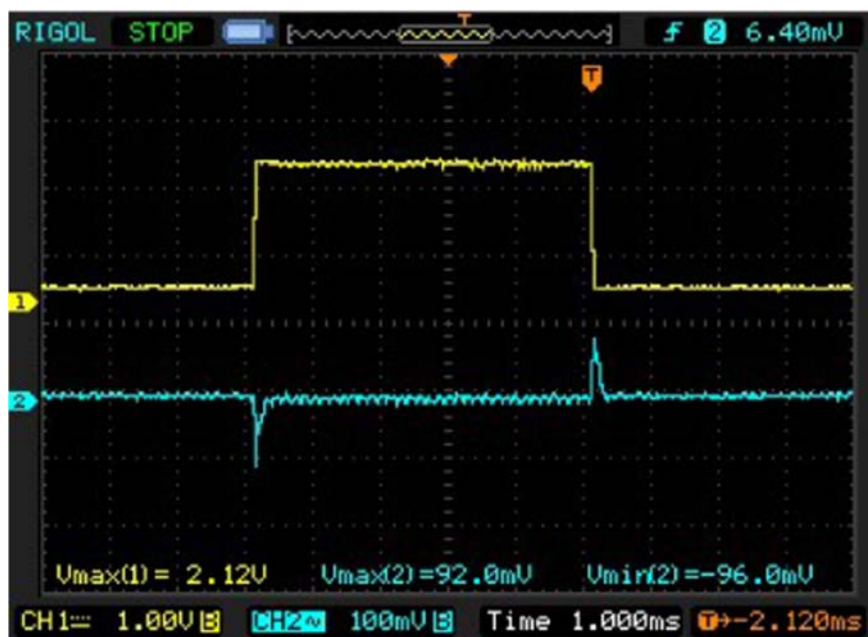
Figure 10. Transient response when load steps from 200mA to 2A in DCM MODE.
