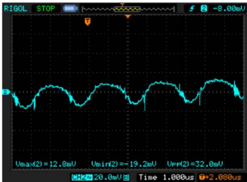
Figure 3. Output ripple at 8A load.
