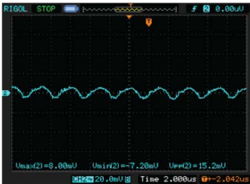
Figure 3. Output ripple at 2A load.
